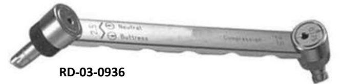
RD-03-0934 DCP Drill Guide 3.5 For neutral a load position, drill bit 2.5m dia.
